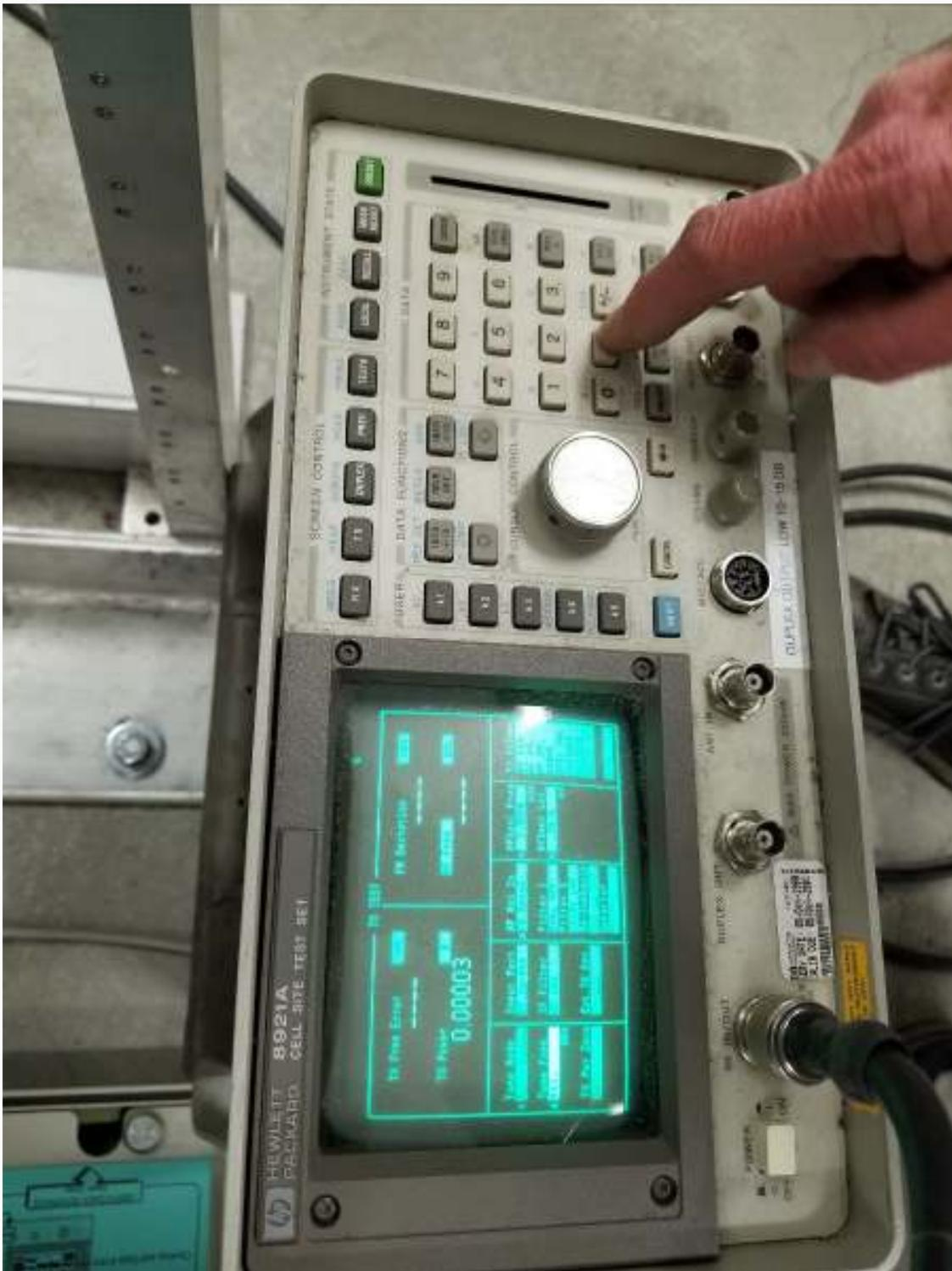
Service monitor in action. It provides a signal which is processed through our equipment, then looks at that same signal to make sure it meets all FCC requirements
